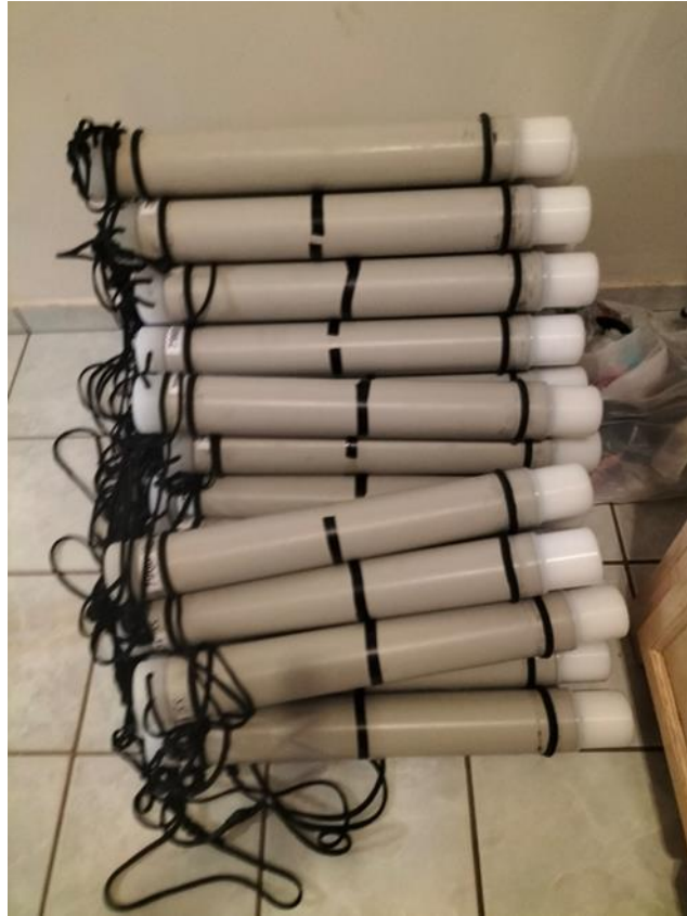
Figure 5. Acoustic detectors F-POD ready for the first deployment in the sampling sites.
