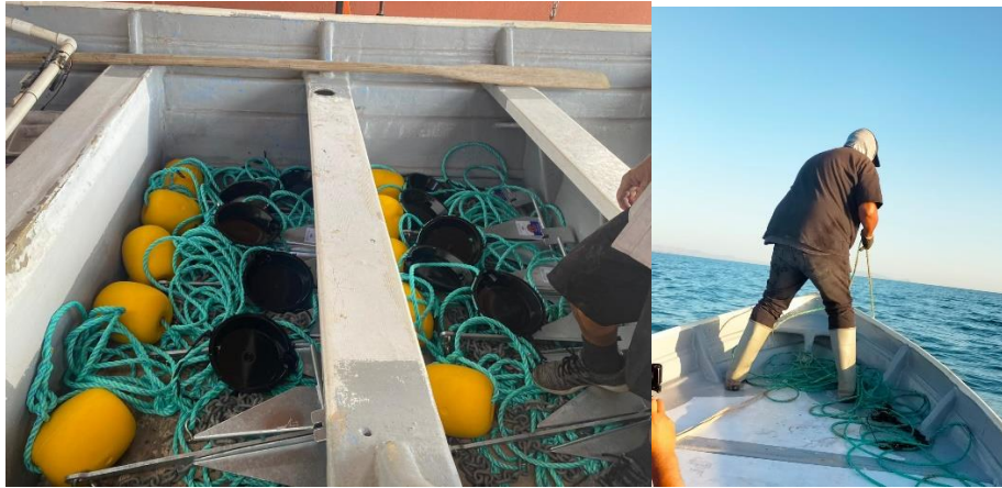
Figure 6. Moorings placed on pangas ready for deployment and Fisher deploying a mooring with acoustic detector.
